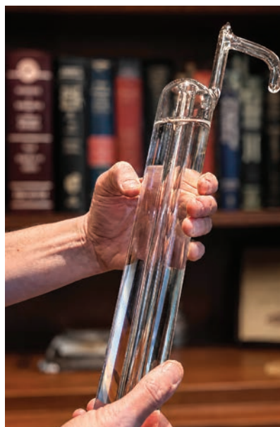
A water triple-point cell. Before the 2019 revision of the SI, the kelvin was defined through the triple point of water. It remains a defining fixed point of ITS-90, with T_{90} = 273.16 K and t_{90} = 0.01 °C. Image credit: Isotech.
